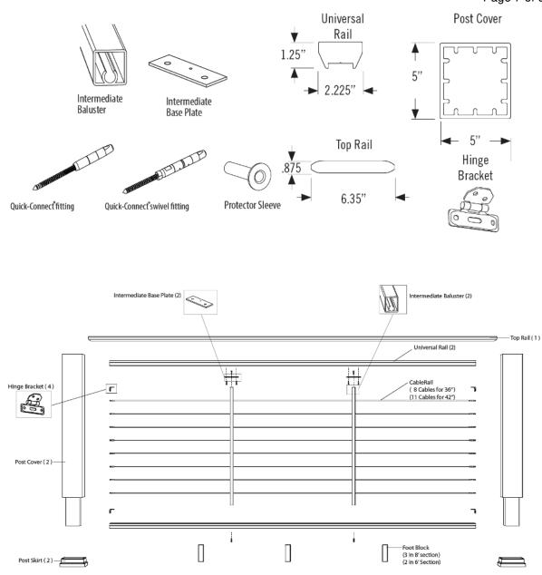
Figure 2 – Evolutions Rail™/ Contemporary with Feeney® CableRail®
