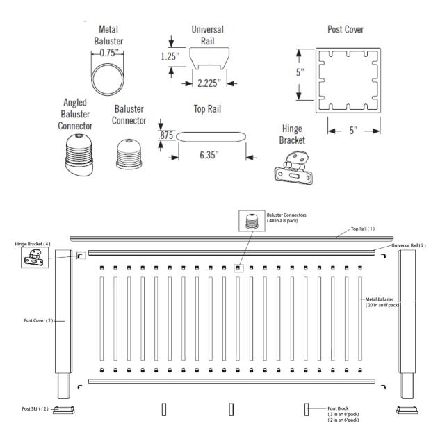
Figure 3 – Evolutions Rail™ / Contemporary with Steel Balusters
