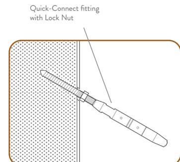
Quick-Connect fitting with Lock Nut
