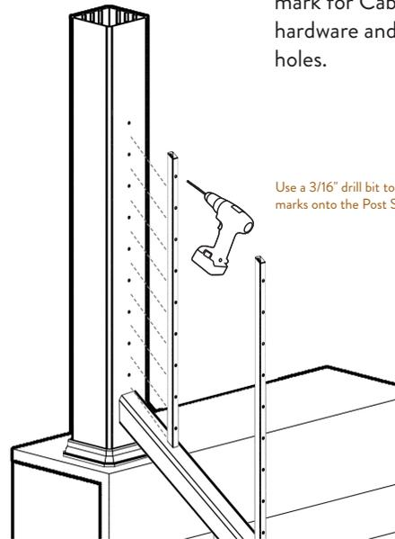
Use a 3/16" drill bit to transfer marks onto the Post Sleeve
