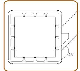
For angled rail installations, align angled face of Support Block parallel to rail section.
