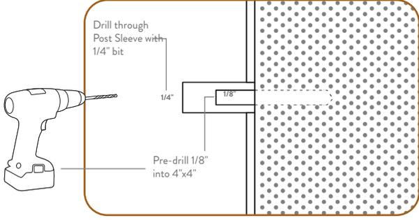
Drill through Post Sleeve with 1/4" bit
