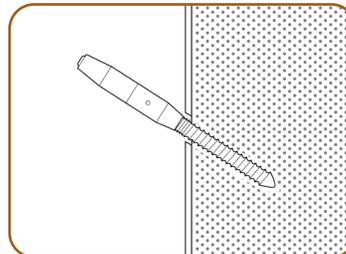
On the side with the lock nuts, screw on the Quick-Connect fittings after the lock nuts, onto the hanger bolts
