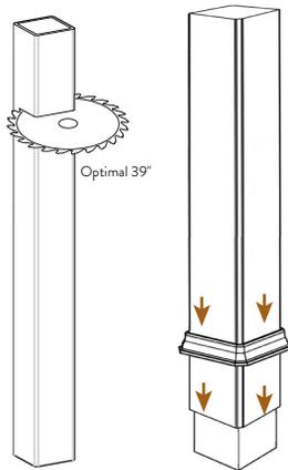
39" above deck surface is optimal for 36" railing heights.
