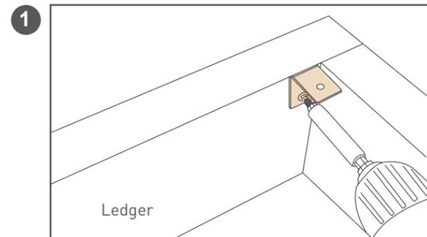
Use the 1-1/2" joist screw provided to install the L-Bracket into the inside of the rim joist.
