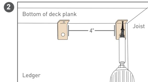
Then use the 3/4" plank screw to attach the L-Bracket to the underside of the plank.
