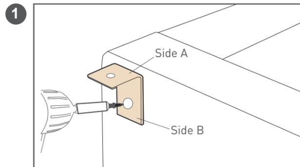
Use the 1-1/2" joist screw provided to install the L-Bracket into the outside of the rim joist.
