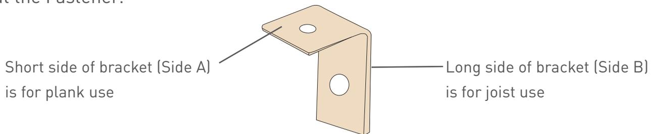
**Clip Spacing:** For either installation option, locate and install one L-Bracket at the start and end of the plank in the corner where the joist meets the rim joist. Then install two clips in every joist bay spaced where  $x = J/2$  and  $y = J/4$  where [J] is the center to center spacing of the joist.
