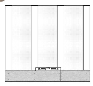
• Choose the starting location of the first course. Position the board with the tongue facing up and ensure it is level prior to fastening.
