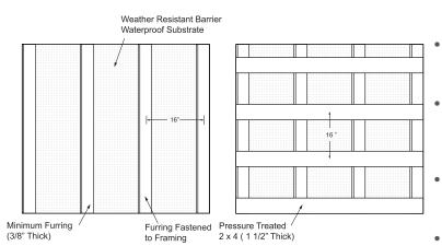
• First, attach the 3/8" thick weather-resistant furring strips vertically over a WRB or weather-tight wall (furring width minimum 1 ½").
